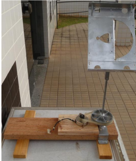
Figure 16 – Prototype with the motor and fixed on wood support.
