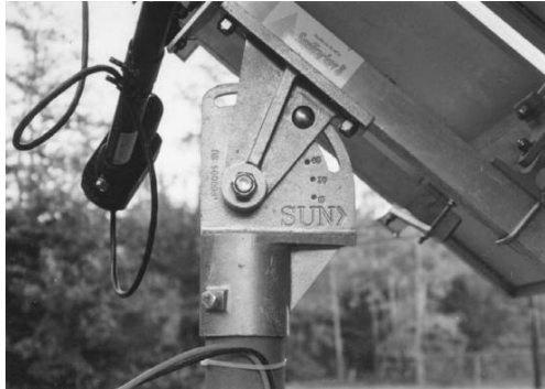
Figure 8 - Parts of one-axis sun tracker [12].
